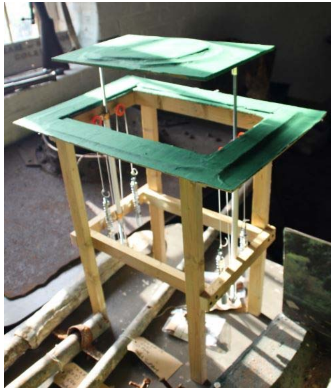
A model example of the vertical rising counterweighted hatch mechanism. © CART.
